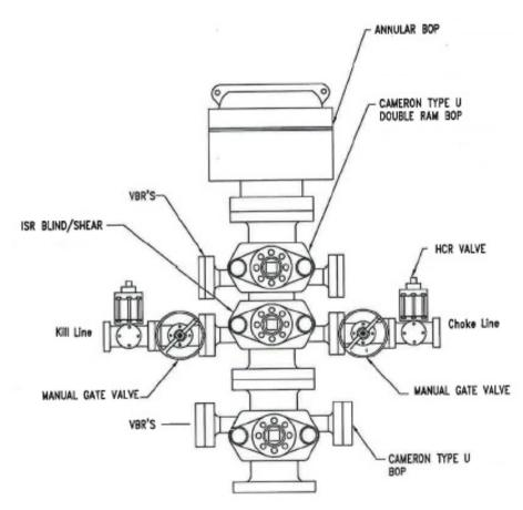
The BOP stack is placed near the top end of the drill pipe. As can be seen, the BOP at issue in this case contained an annular BOP, a double ram BOP, and a single ram BOP. The annular BOP is used to seal the space around the
