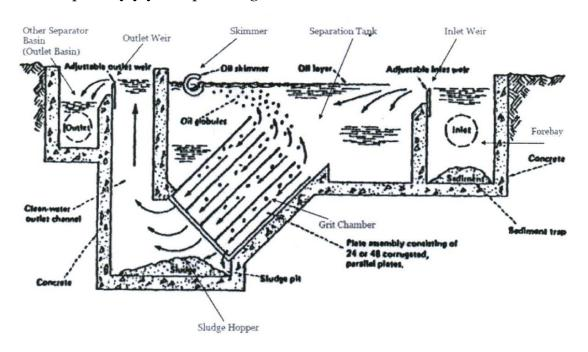
Notably, the definition in Subpart QQQ exactly describes this diagram. All of the components listed in Subpart QQQ (separation tank, forebay, other separation basin, skimmers, weirs, grit chamber, and sludge hopper) are identifiable on the diagram, and they are components of the separators as described by EPA. *See* Background for Proposed Standards, *supra*, at 3-30.
